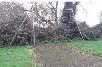
**Finding:** The surfacing width under the seat/s is / are less than 875mm when measured from the centre of the seat outwards, and fails the requirements of BS EN 1176 Part 2
