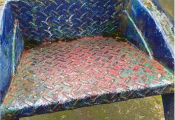
**Finding:** The paintwork on this item has been damaged or worn exposing the metal underneath which is rusting / corroding
