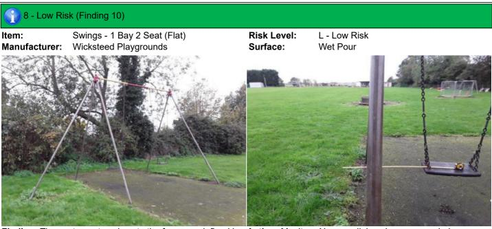
**Finding:** The seats are too close to the frame as defined in BS EN 1176 Part 2; this is a low risk failure and no remedial action is required
